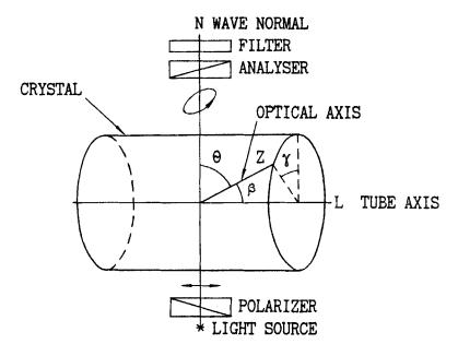
FIGURE 1 Schematic drawing of the optical system.
